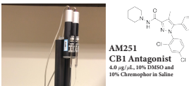
Figure 9: Custom designed injection rig. This rig was designed to infuse drugs into the brain via a cannula system in an awake mouse. Anesthetic agents such as isoflurane can interfere with olfactory perception which created the need for this custom injection rig. Mice were infused with 1.0 µl per MOB at 100 nM per minute. Mice were given 10 minutes before the infusions were removed from the gait cannula then 20 minutes in their home cage prior to behavioral testing.
