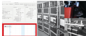
Figure 7: Images of our semi-automated, Arduino-controlled, head-fixed, behavioral rig setup and flow dilution olfactometer. Mice were first acclimated to head fixation and trained to lick for water. Mice were then trained to discriminate between the isoamyl acetate odor and the mineral oil solvent.
