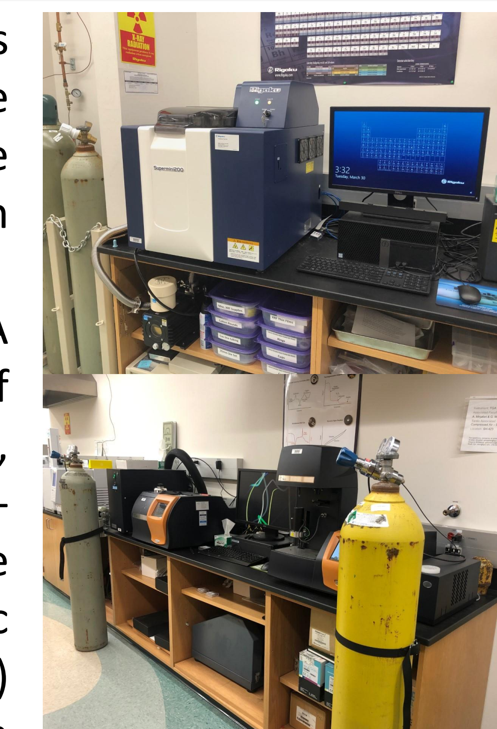
Figure 1. Rigaku Supermini200 WDXRF (top) and TA Instruments DSC 250 and TGA 550 (bottom).
