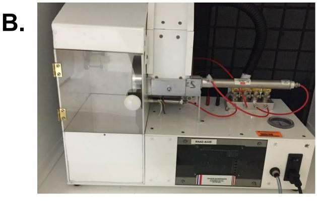
**Smoke exposure apparatus.** Rats were placed in standard home cages, which were placed into the upper chamber of the exposure apparatus (brown-tinged chamber in A.). Cigarettes were burned sequentially using an automated smoking machine (B.) from which the smoke was pumped into the exposure chamber.
