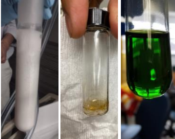
Figure 3. CSC in the condenser (left), final CSC concentrate (middle), and cannabis plant extraction (right).
